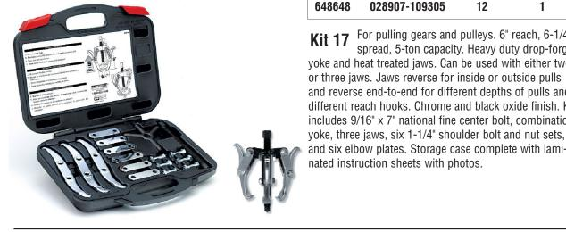
Kit 17 For pulling gears and pulleys. 6" reach, 6-1/4" spread, 5-ton capacity. Heavy duty drop-forged voke and heat treated jaws. Can be used with either two or three jaws. Jaws reverse for inside or outside pulls and reverse end-to-end for different depths of pulls and different reach hooks. Chrome and black oxide finish. Kit includes 9/16" x 7" national fine center bolt, combination
