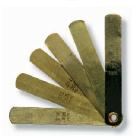
For adjusting air gap clearances on some types of electronic ignition systems. Gauge set contains non-magnetic brass blades. Blades include: 0.006, 0.008, 0.010, 0.012, 0.014, 0.016. Meets Fed Spec. GGG-G-17c.
